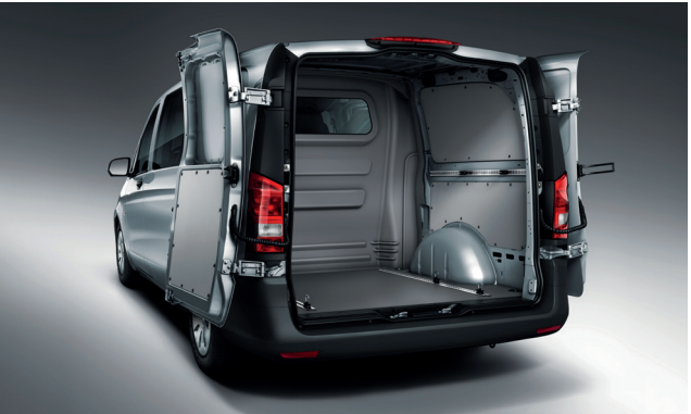
● The full-width partition wall with window at the C-pillar helps keep the passenger compartment clean and offers additional protection from your cargo. Optional barn doors shown.
