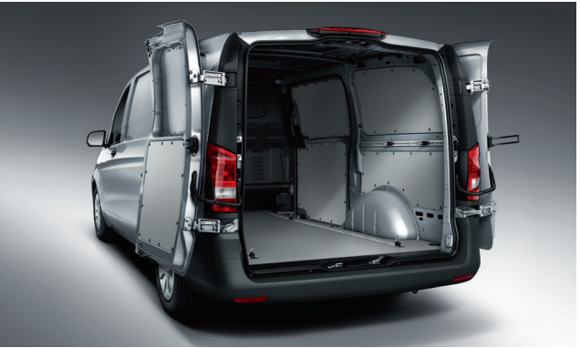
The two (optional) rear doors can be opened back to the side walls and secured, making loading and unloading easier. Optional equipment shown.
