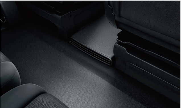
● The air-duct to the passenger compartment provides the rear passengers with temperature-controlled air.
