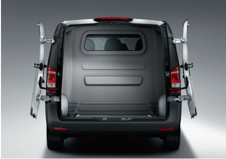
The two rear barn doors can be opened back to the side walls and secured, making loading and unloading easier.
