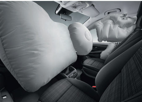
The dual front airbags and curtain airbags for driver and co-driver form part of the extensive range of standard-fit safety equipment. The optional thorax-pelvis sidebags in the front offer additional protection.
