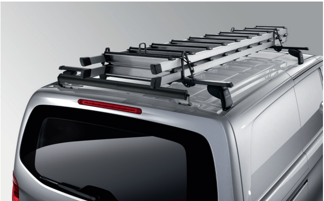
Set of two basic carrier bars, screw-fit to designated points in roof channel. Adding an optional 3rd crossbar increases maximum permissible roof load from 100 kg to 150 kg. Optional ladder rack attachment and loading roller attachment also shown.
